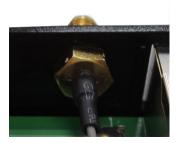
5. Install the connector; place the locking washer first, and then tighten the nut. Locking Washer
