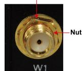
6. Connect the antenna to the connector.
